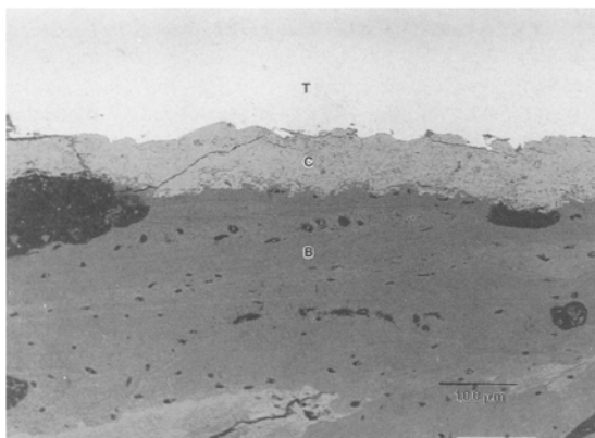
Figure 1 SEM photomicrograph of a titanium (T) implant with a hydroxylapatite (C) coating after several months of implantation in a human jaw. Bone is B; darkest areas are epoxy potting compound.
